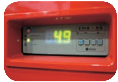
Energy management devices detect the opening hours of a store and adjust the cooler's temperature. They turn off lights and reduce fan operation thereby saving up to 35% energy use.
